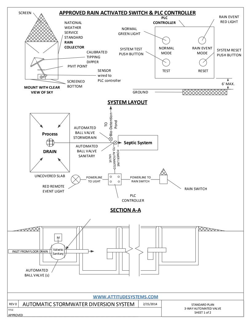
1. THE RAIN SWITCH WILL PROVIDE A SIGNAL TO THE AUTOMATED VALVE TO SHUT OFF ACCESS TO THE SEPTIC SYSTEM AND OPEN ACCESS TO THE BIO-DETENTION POND AFTER 0.1" OF RAINFALL OVER ANY CONTINOUS 60 MINUTE PERIOD.
