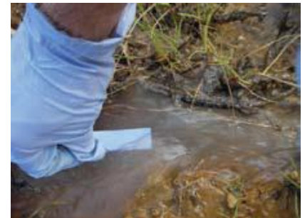
A Hydrocarbon Detection Strip is used to monitor the filtered water leaving the EVAC Filter.
